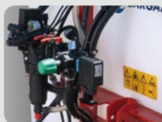
Electric control unit with electric valves
