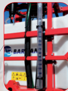
Top water level checking accuracy in the tank via a dry graduated scale
