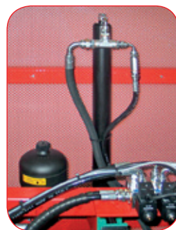
Gas accumulator on lifting piston (◉ optional on BDU and BDU PLUS)
