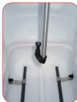
Rotating nozzles for internal cleaning of the main tank (◉)
